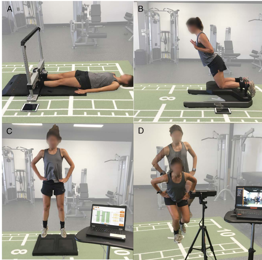
FIGURE 1 —Demonstration of the strength and biomechanics field-based testing battery. A , Isometric hip adductor and abductor strength. B , Eccentric knee flexor strength during the NHE. C , Bilateral CMJ on portable force plates. D , Single-leg triple vertical hop kinematics using a markerless motion capture system.
